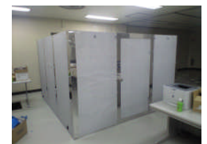
Light Anechoic Chamber
