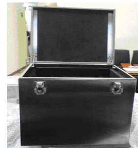
Shield Box with millimeter wave absorber
